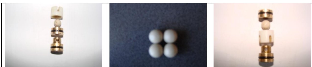
Fig.18 a-Supapa aspiratie; b-Bile; c-Supapa refulare
